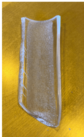
Figure 4.3: Picture of the fine grained plastic particles used to emulate borehole wall roughness that covers the lower side of the PMMA tube
