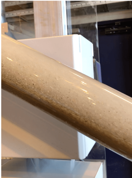
Figure 5.4: Picture illustrating sand particles being carried in suspension during the loading procedure using the 0.2 wt-% xanthan gum fluid.
