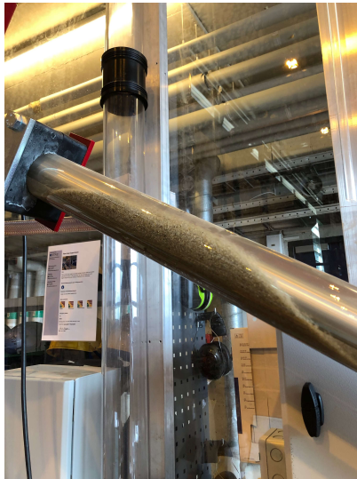
Figure 5.2: Picture of the upper part of the test tube during a circulation only test run illustrating how the cuttings bed moves in the absence of drillstring rotation
