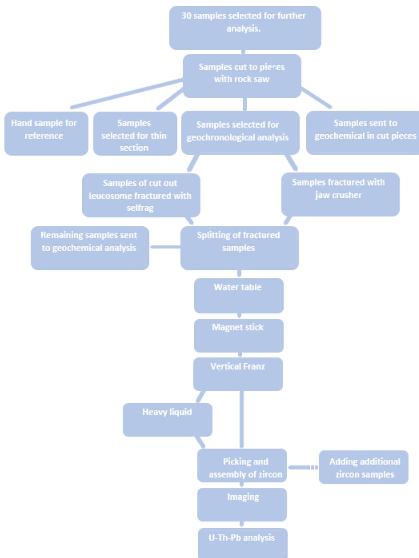
Figure 4.2: Workflow diagram for sample analysis
