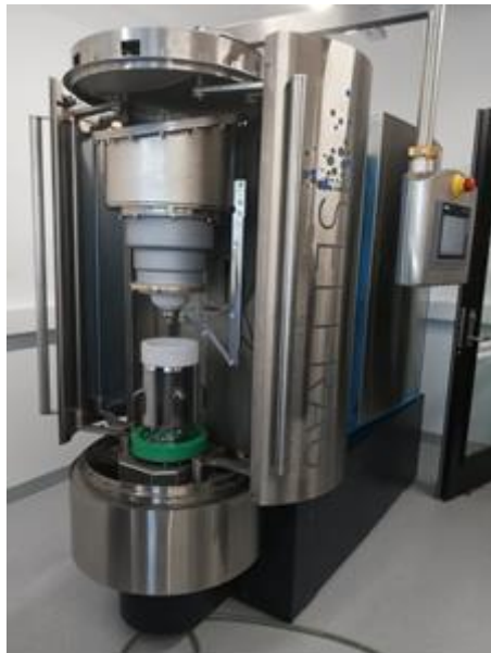
Figure 4.3: SelFrag Lab at NTNU. The sample container can be seen on the green holder in the machine.
