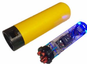
Figure 3.3: Capsule and instrumentation of a Sensorfisk, (SINTEF Ocean, 2019)
