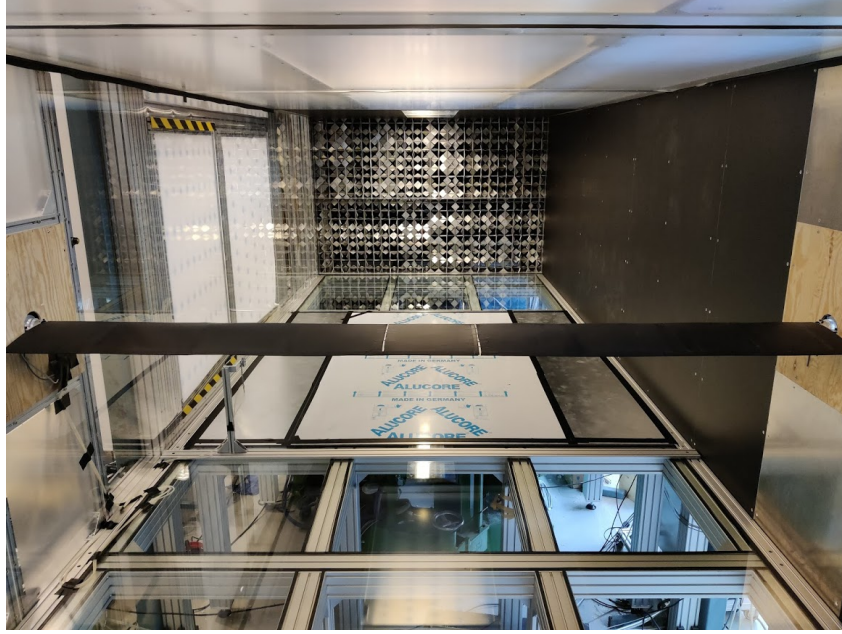
Figure 2: Airfoil mounted to the load cells and forced vibration rig in the test section. Also visible: the active turbulence grid in the background, the Pitot-static tube under the airfoil on the left side, and the thermocouple on the right wall, just under the airfoil section.
