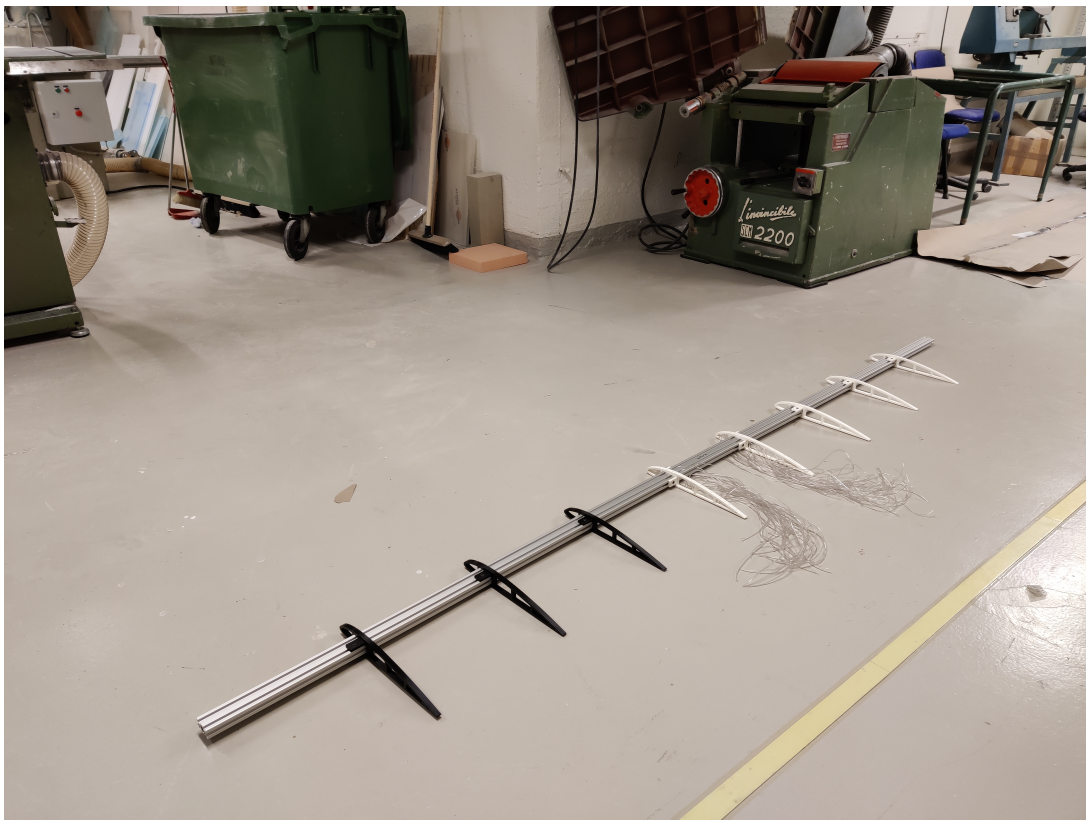
Figure 21: Mounting of the ribs to the spar
