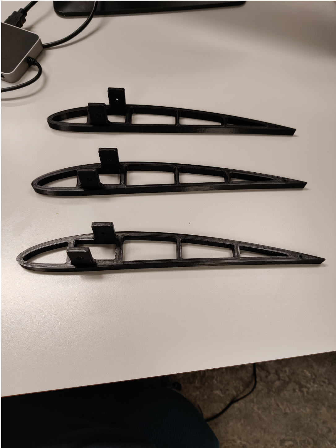
Figure 20: NACA4412 ribs with mounts to the spar
