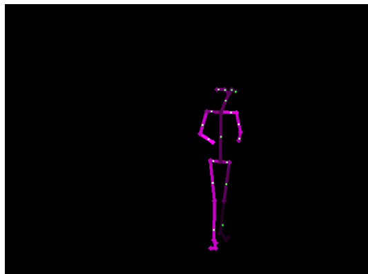
Fig. 4. Centroids of all parts are shown in green color where the skeleton is shown in pink.
