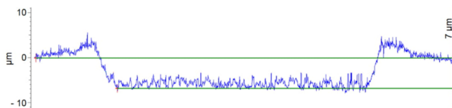
Figure S3: Flat crater profile for tantalum with small grains at discharge condition of 2.3 mA, 0.7 kV using 0.25 ml/min argon flow after sputtering for 1.5 h, zoomed with a different axis scale using Figure 1B.
