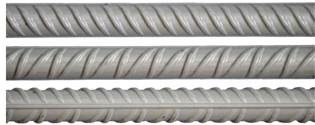
Fig. 6 The rebar bolt used in these tests: 20 mm in diameter, made of type B500NC steel and corrosion protected with hot galvanising and powder coating
