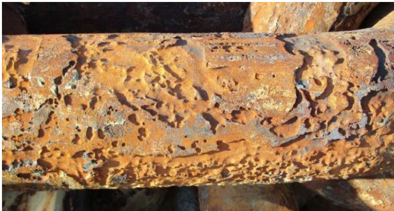
Figure 21: Characteristic worst case pits made from MIC/SRB [38]
