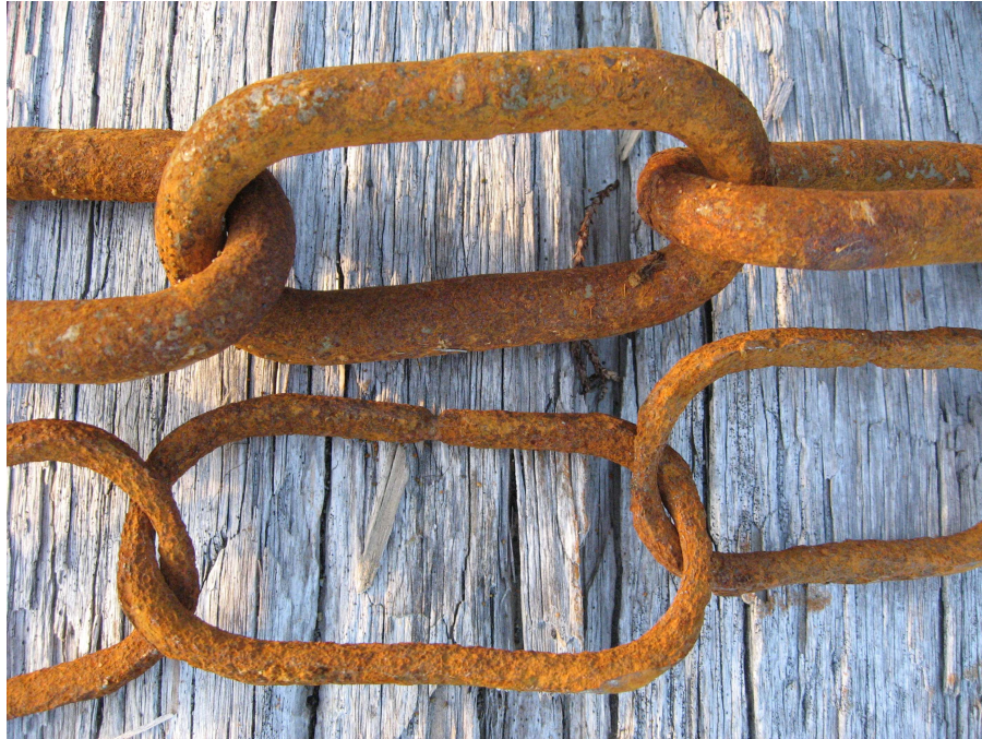
Figure 16: Chains with varying degree of corrosion[35]
