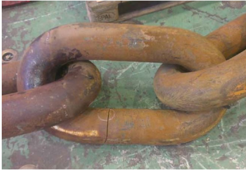
Figure 33: Link with failure in wear dent. Break in white circle. [22]
