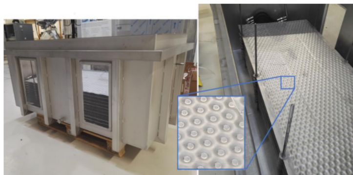
Figure 53: CTES unit NTNU LAB [70]
