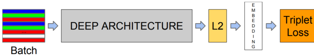
Figure 15: Model Structure for FaceNet [60]
