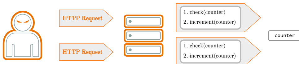
Figure 4.1: The attacker sends two parallel requests that get served concurrently by two threads. Both threads read and later increment the counter, leading to a potentially different result as when the requests would have been executed sequentially.
