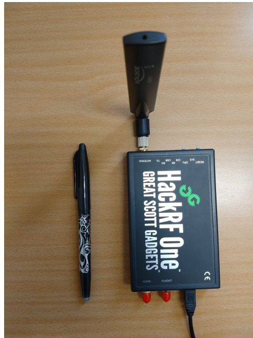
Figure 5.1: HackRF One with a pen next to highlight the size of the device
