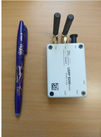
Figure 4.1: A USRP B200mini with a pen next to highlight the small size of the device
