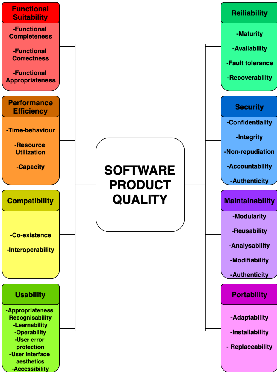
Figure 3.1: Illustration of characteristics and associated subcharacteristics from ISO/IEC 25010:2011.
