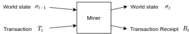
Figure 2.12: Executing a Ethereum transaction to produce a new world state and transaction receipt.
