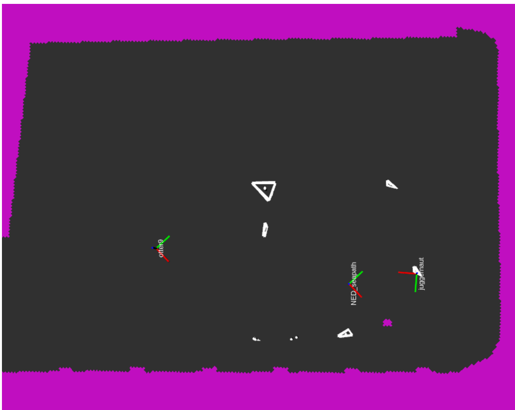
Figure 49: The output from Euclidean clustering and land filtering.
