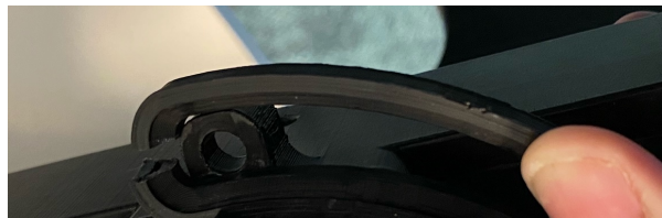
Figure 44: The broken camera mount.
