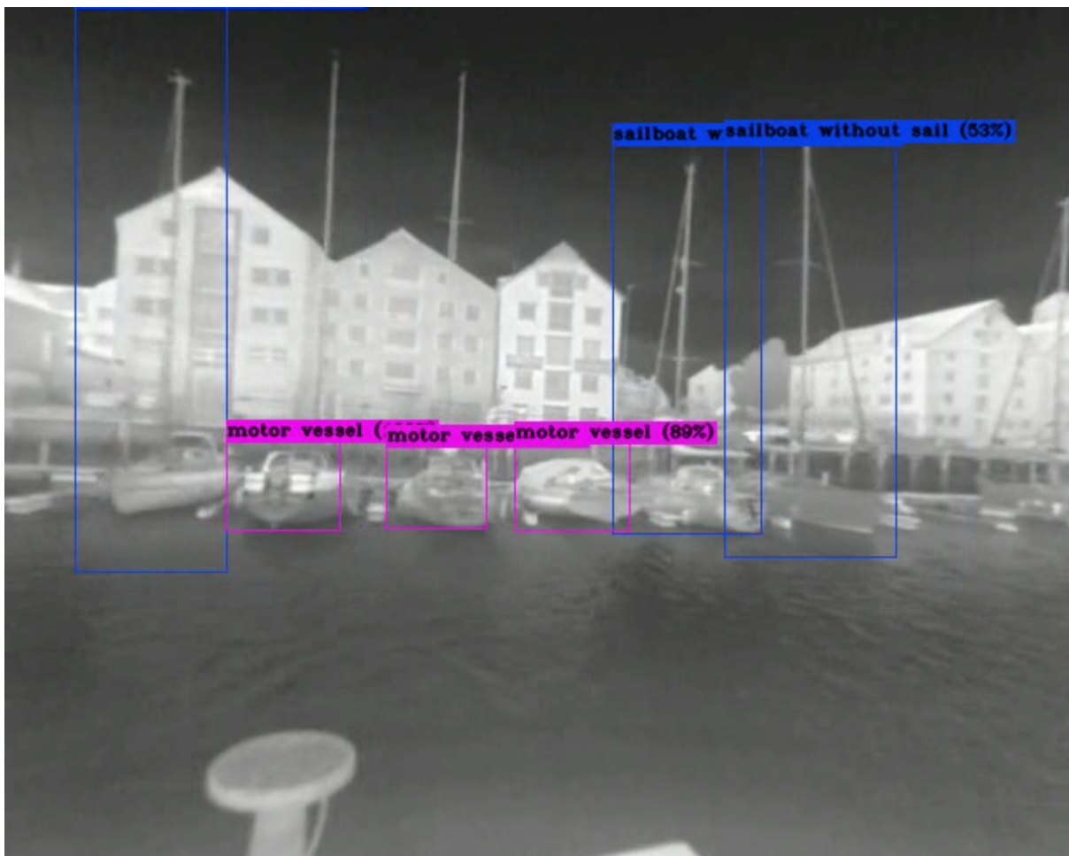
Figure 2: Object detections with YOLO V3 using an IR-camera.
