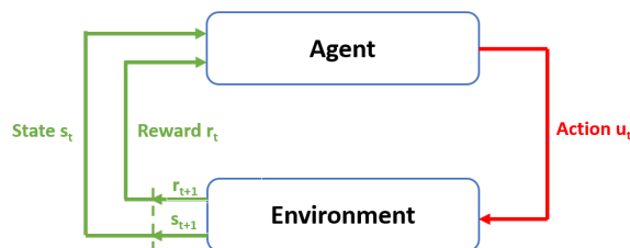
Figure 4.1: A flow diagram describing the general framework in reinforcement learning.
