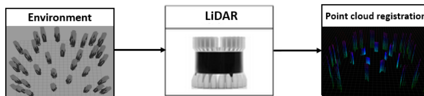
(b) An environment perceived by a LiDAR registering a point cloud.
