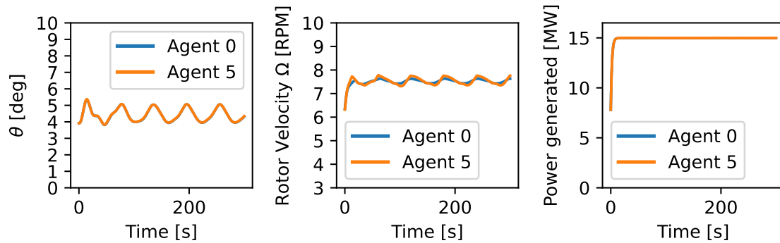
(b) Response for wind mean 16 m/s and amplitude 3 m/s, with a PSF.
