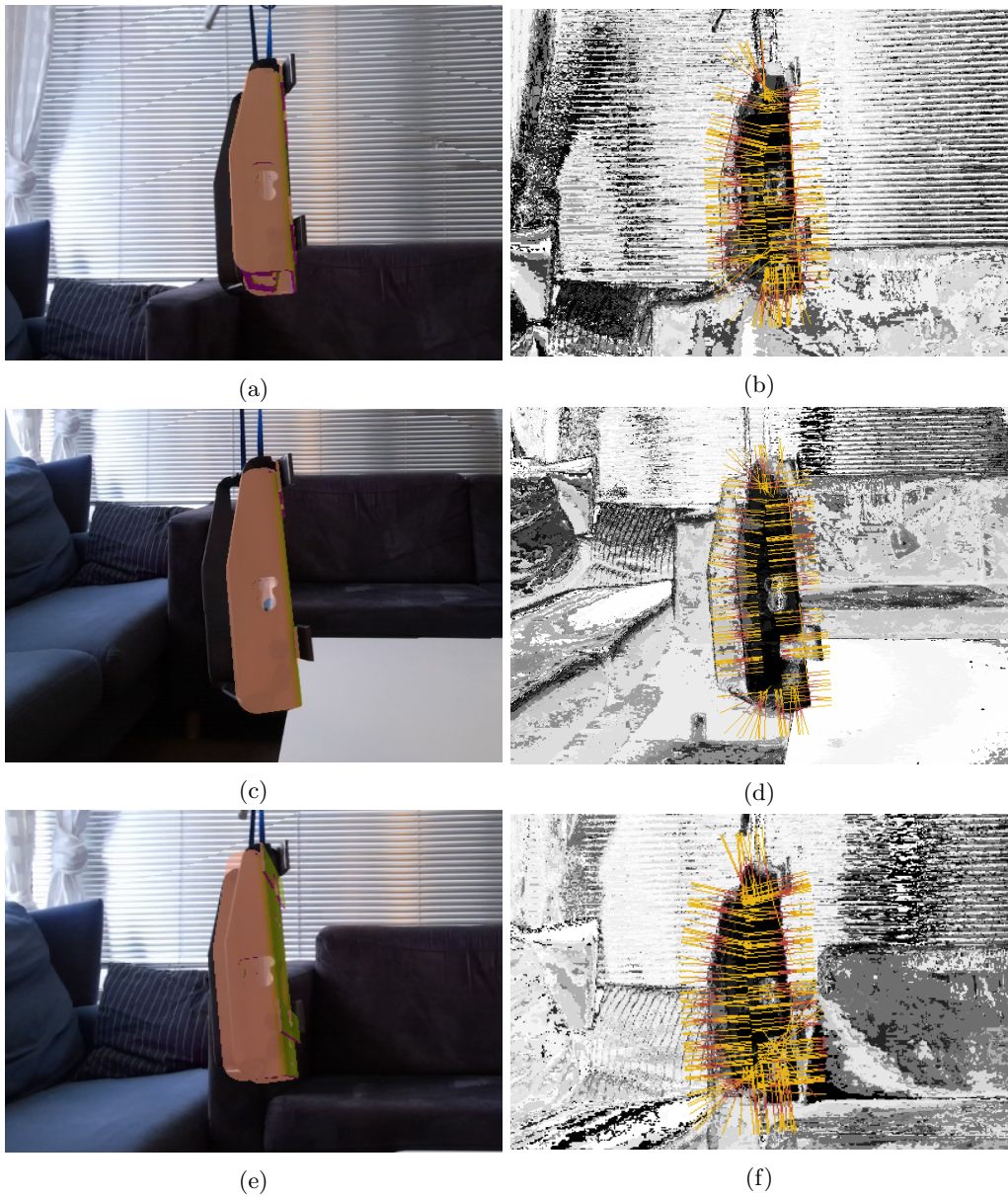
Figure 39: Samples from a tracking run using the original RBGT method [48]. Incorrect appearance models and corresponding posteriors causes the tracker to misinterpret the object’s rotation in a) - d) . In e) and f) the imprecise nature of the contour likelihoods lead the tracker to pick out the opposed pose variation.
