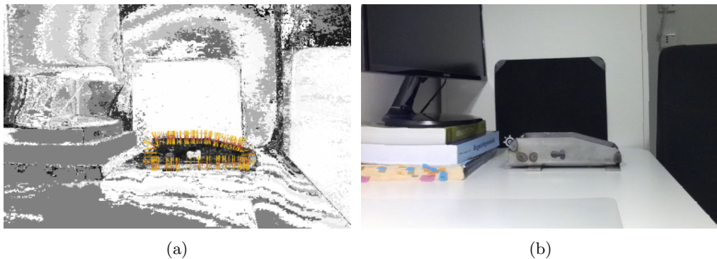
Figure 18: Sample of posterior membership probabilities given a RGB image and color histogram models p(\mathbf{y}|m_f) and p(\mathbf{y}|m_b) . a) Pixel-wise posteriors describing the probability of a pixel belonging to the background. White pixels indicate p_b = 1 , while black pixels indicate p_b = 0 . When updating the color histograms, the method uses RGB values along the orange correspondence lines. The line segments with high contour probability are indicated by red. b) Corresponding RGB input image.
