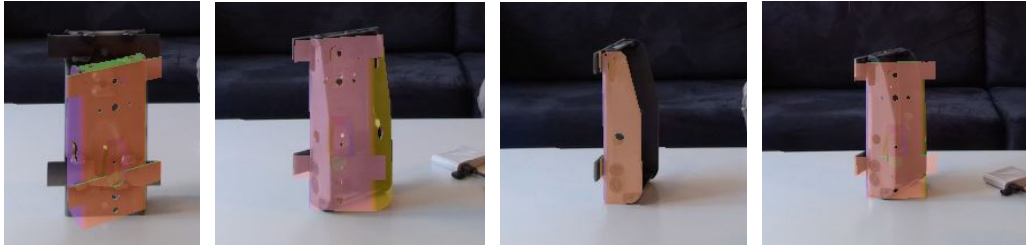
Figure 46: Examples of inaccurate pose estimates with low variance scores due to contour ambiguity and a lack of trustworthy depth based likelihoods.
