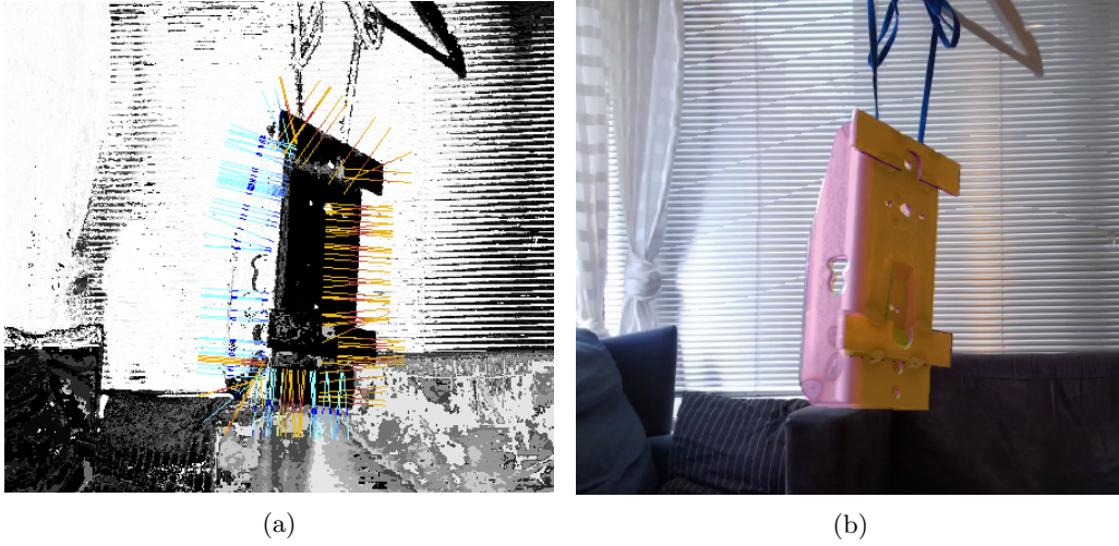
Figure 38: Example demonstrating the impact of utilizing depth information. a) The pixel-wise posteriors indicate p_b \approx 1 for the leftmost part of the object. However, the depth based likelihoods make sure that the tracker maintains the correct pose estimate. b) The resulting pose estimate.
