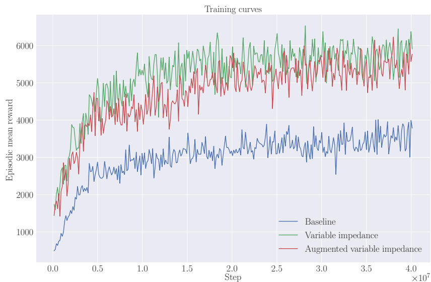
Figure 5.1: Training curve for each of the three models. The curves show how the models learn as they are being exposed to more simulation data. The baseline model is used as a reference to quantify the effect of using an appropriate low-level controller.
