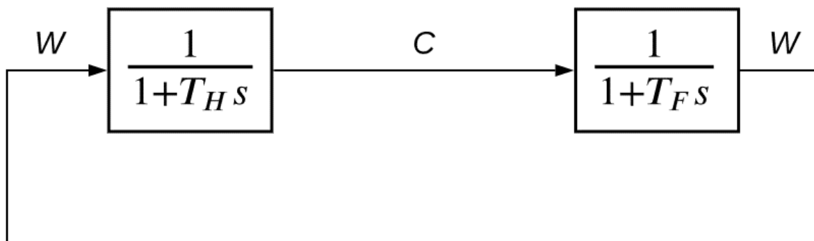
Figure 3.7: Simplified block diagram of the firm-household-system, where W is wages and C is private consume. Based on figure 2.16 in (Andresen, 2018, p. 34).
