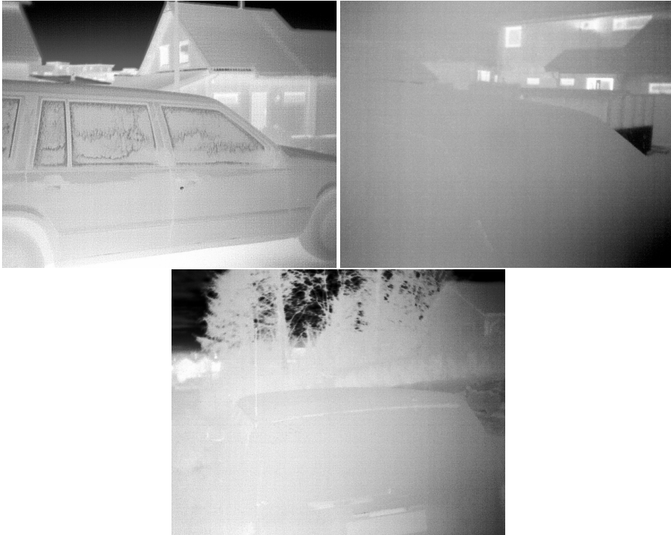
Figure 6.9: A cold car, with approximately the same temperature as its surroundings. The upper left image is before snowfall, while the following two images are after snowfall has laid an approximately 2 cm coat with very even temperature, making the car almost invisible in the thermal images.
