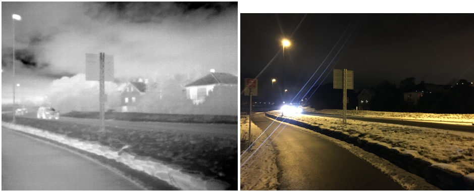
Figure 6.10: How many cars? The thermal camera is not blinded by the car lights, making it easier to spot and count the cars.
