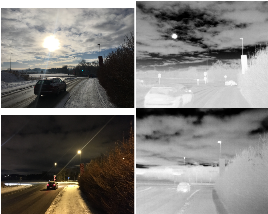
Figure 6.11: Well lit intersection. The thermal camera provides very similar images both day and night, and is not blinded by the sun.
