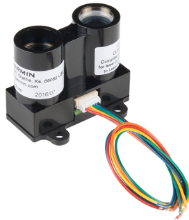
Figure 2.8: The Garmin lidar v3 sensor, image from Sparkfun [33]
