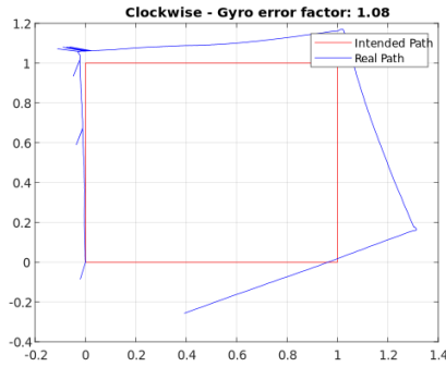
Figure B.2: Square test result with gyro error factor implemented
