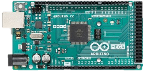
Figure 2.2: Arduino ATmega 2560, image is taken from the Arduino homepage [21]
