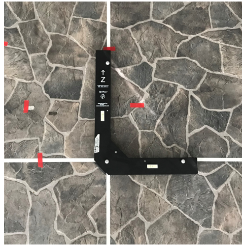
Figure A.4: Placement of the calibration L in the testing area
