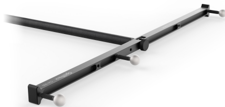
Figure A.3: Wand used to calibrate the Optitrack camera, image from [46]
