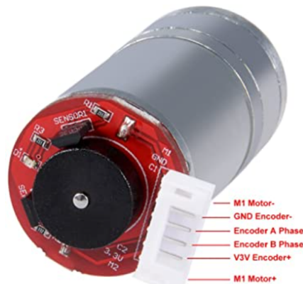
Figure 2.13: Connector sheet for the new motor and encoder, image is from [49]
