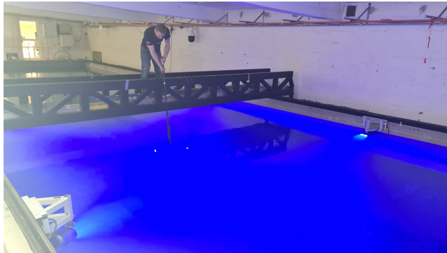
Figure 6.7: Qualisys underwater camera system physical calibration setup
