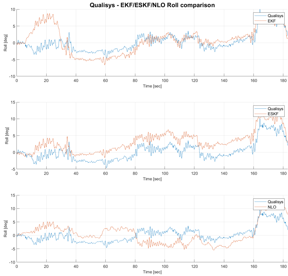
Figure 7.70: Roll comparison between the EKF, ESKF and NLO compared to Qualisys - underwater square
