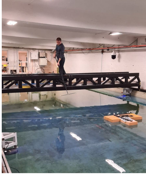
Figure 6.4: Qualisys "above water" calibration volume setup
