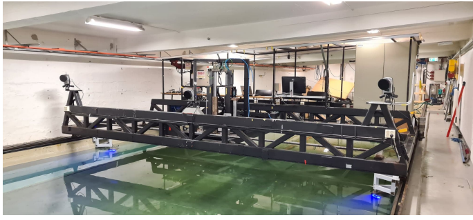
(a) The Marine Cybernetics testing basin and the Qualisys camera locations
