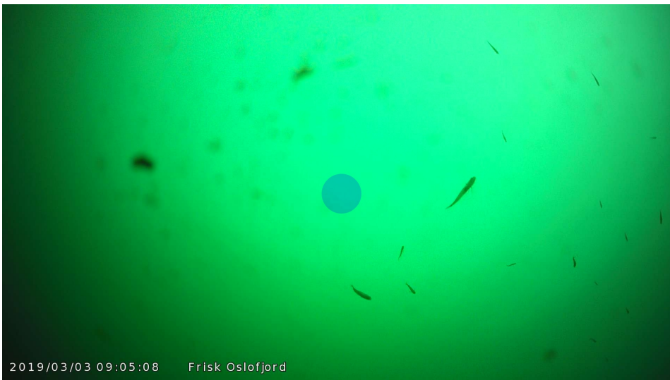
Figure 4.2: Illustration of the sonar region within an image. The blue circle is observed by both the optical and the acoustic sensor.
