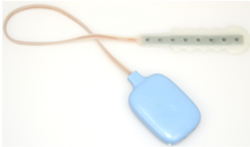
Figure 3.1: The vaginal pressure sensor, called FemFit, used to collect the dataset.
