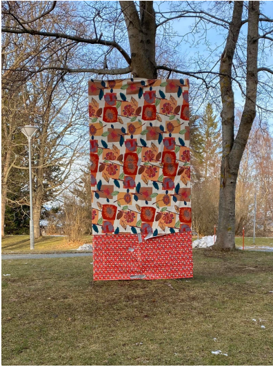
(a) Object for LiDAR-stereo camera calibration
