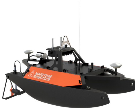
Figure 1.2: Picture of the Otter USV. Illustration from Geo-matching (2019)
