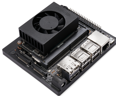
Figure 4.1: Jetson Xavier NX Developer Kit. Image courtesy of Nvidia (2020).
