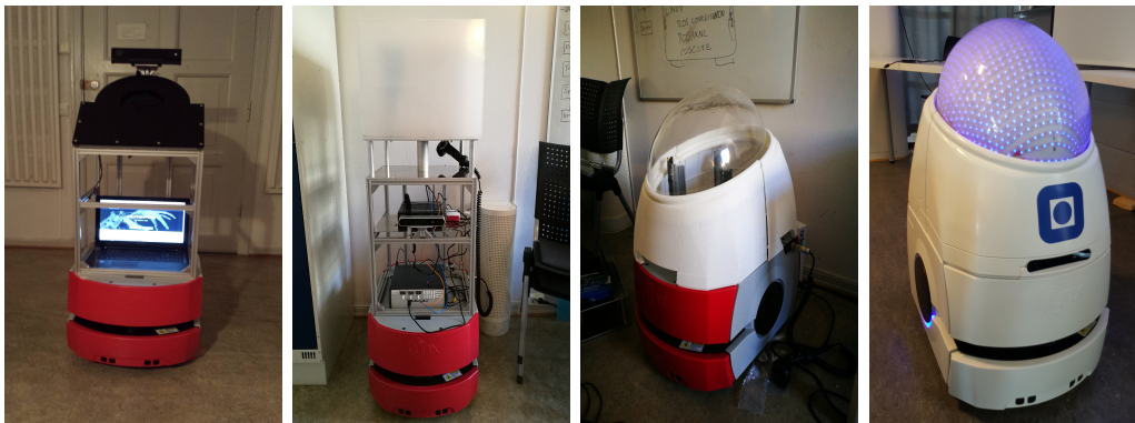
(a) 2016: Skeleton frame (b) 2017: Selfie stick, Kinect (c) 2018: 3D printed casing (d) 2019: Dome, paint-job
