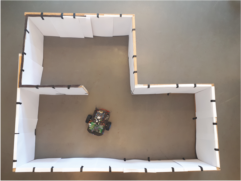
Figure 12.5: Labyrinth track used to test slam.
