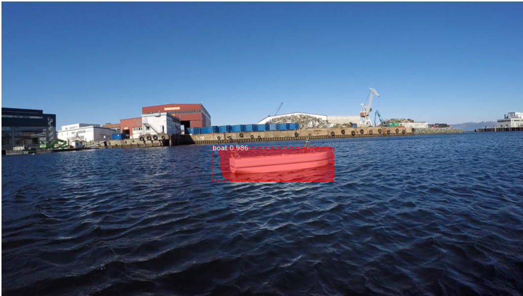
Figure 5.22: Mask R-CNN model trained in the simulated environment tested on Image 1 with the boat class prediction of 0.986.
