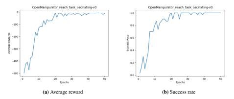
Figure 5.12: Success rate and average reward from training one agent on the reaching task with oscillations in PyBullet
