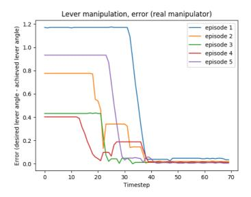
Figure 5.11: The error on the real world manipulator on lever manipulation task
