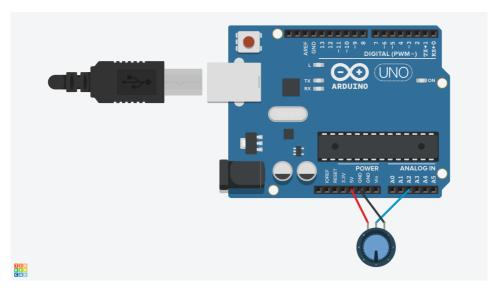
Figure 3.3: Potentiometer setup with Arduino Uno. Image is made using Tinkercad [6].
