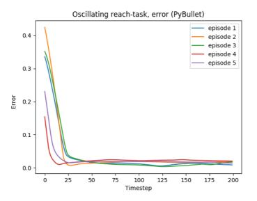
**Figure 5.13:** A plot of the euclidian distance from the end-effector to the goal for five episodes for an agent that has finished its training on the reach-task with oscillations in PyBullet.
