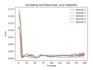
**Figure 5.15:** A plot of the euclidian distance from the end-effector to the line for five episodes for an agent that has finished its training on the line following-task with oscillations in PyBullet
