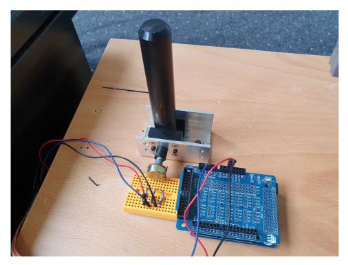
Figure 3.4: The lever, arduino and potentiometer setup
