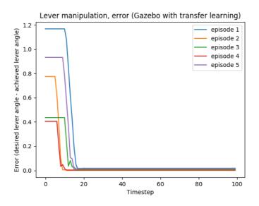
Figure 5.10: The error in Gazebo after transfer learning on lever manipulating task
