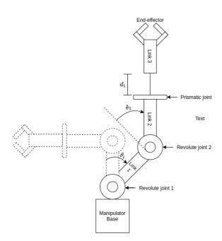
Figure 2.10: Illustration of a Revolute-Revolute-Prismatic (RRP) manipulator
