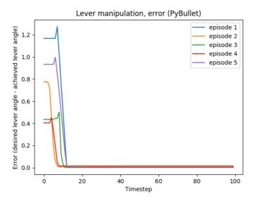
Figure 5.8: The error in PyBullet on lever manipulating task
