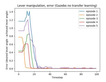
Figure 5.9: The error in Gazebo before transfer learning on lever manipulating task
