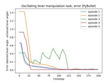
Figure 5.17: A plot of the distance between the achieved lever angle and the desired lever angle over the test episodes
