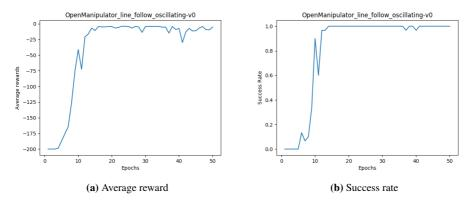
Figure 5.14: Success rate and average reward from training one agent on the line follow task with oscillations in PyBullet.
