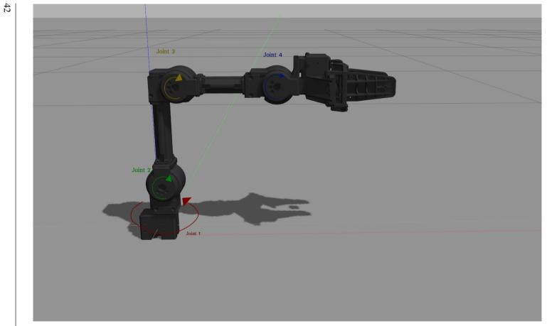
Figure 3.2: Illustration of the joint numbering of the manipulator (screenshot taken in Gazebo)
