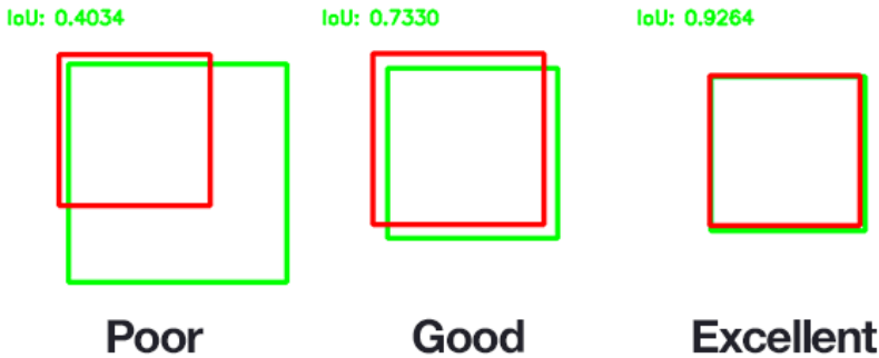
Figure 2.19: Examples of various bounding box predictions and their corresponding IOU scores. The figure is from [16].
