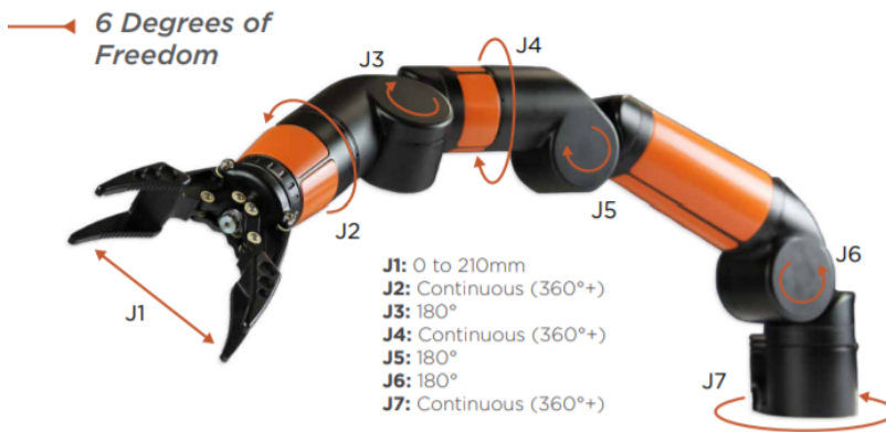
Figure 5.1: Joint definitions of BluePrintLab's Reach Bravo manipulator.
