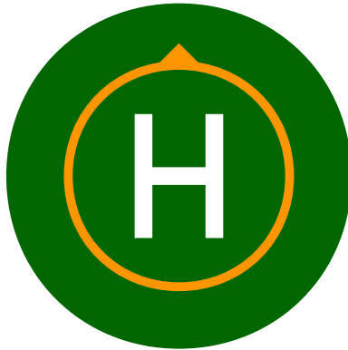
Figure 4.8: The landing platform, also referred to as helipad, seen from a bird's-eye view. The helipad was designed such that the perception module would have the required amount of features to work with for the computer vision modules. The H is of size 0.20 \text{ m} \times 0.28 \text{ m} . The distance from the center of the helipad to the arrow tip is 0.30 \text{ m} , while the radii of the orange and green circle are 0.26 \text{ m} and 0.40 \text{ m} , respectively. Figure courtesy of [39].
