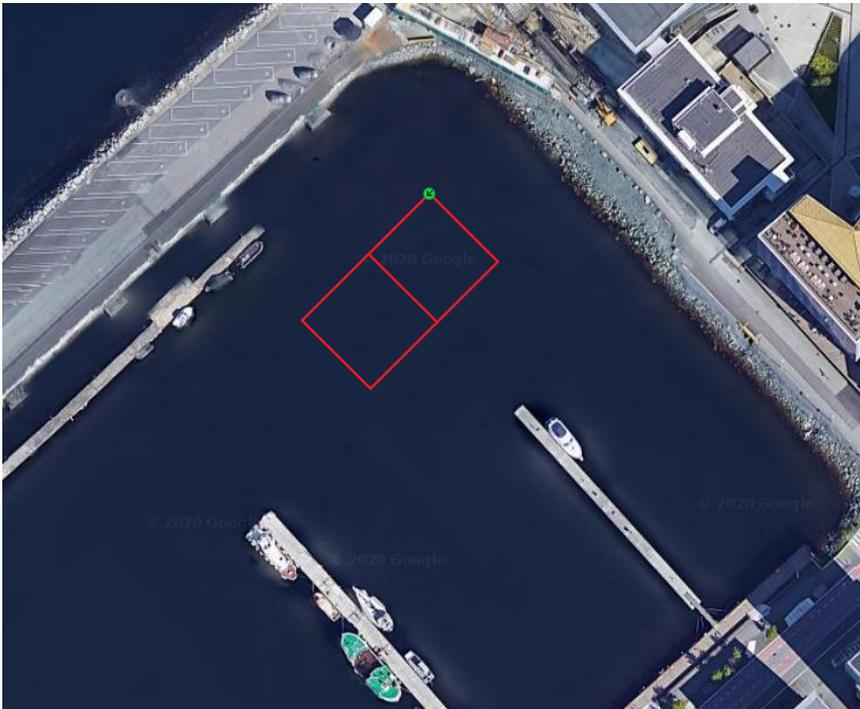
**Figure 5.2:** Path of the experiment in the test area. The starting position of the ferry indicated by the green point. Courtesy of Google Maps.
