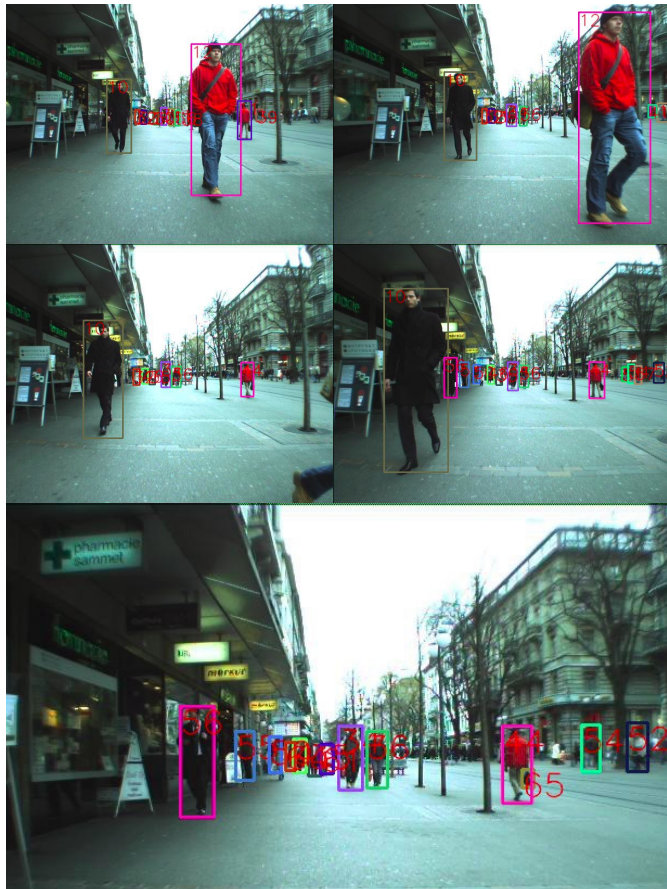
Figure 6.4: Basic SORT algorithm tracking performance on the ETH-Bahnhof data-set with dynamic threshold.
