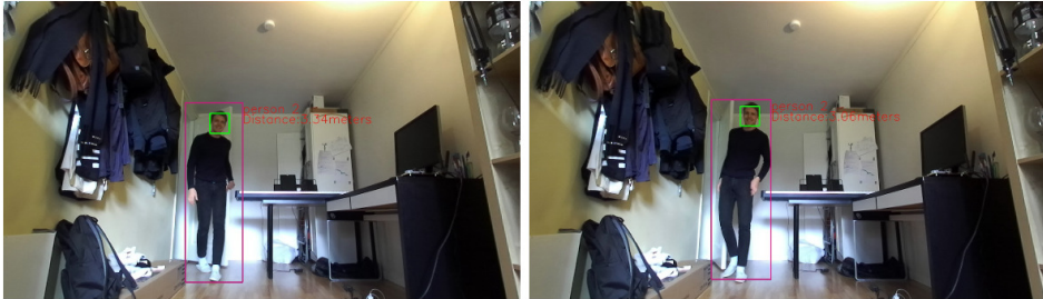
Figure 6.8: Captured result from face and smile detection test, with ZED camera capturing HD720 images.
