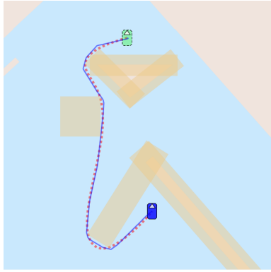
Figure 3.5: Warm-starting: The initial guess created by the A* warm-starting algorithm is shown in blue, while the resulting planned trajectory based on this guess is shown in dotted red. However, as this example illustrates, the shortest path is not necessarily the best. Simpler trajectories could be achieved by adding a cost of being too close to the obstacles both in the A* algorithm and the OCP.
