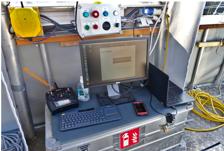
Figure 5.23: The control station of the ship, with screen, keyboard and RC controller.
