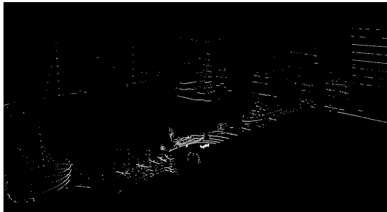
Fig. 2. Point cloud recorded by the ASV (MilliAmpere) before pre-processing the data (7713 points)
