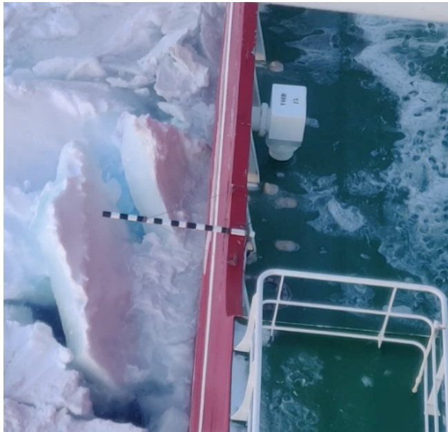
Figure 4.9: The yardstick used to measure ice thickness positioned horizontally from the ship. Each white and black segment is ten centimetres long. The ice thickness shown here is estimated to be approximately 40-50 centimeters.
