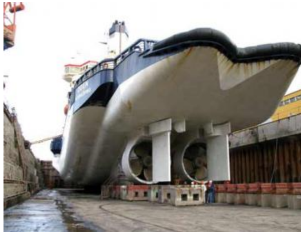
Figure 14: The propellers installed on Oden. Photo: Garay (2007)
