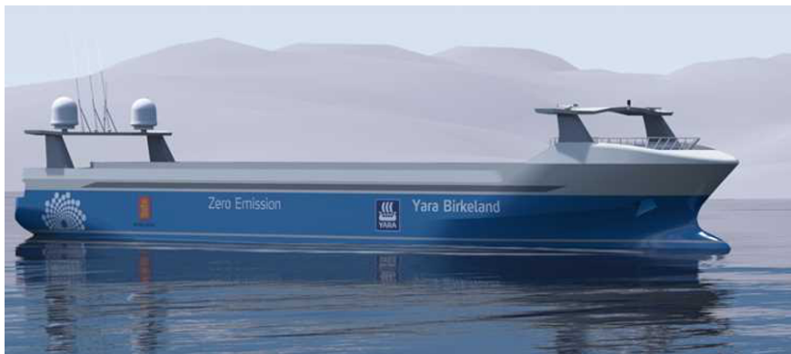
Figure 22: Illustration of Yara Birkeland, the zero-emission autonomous container vessel developed by Kongsberg Maritime for Yara (Maritime 2017).
