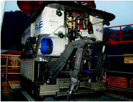
(a) ROV used for trenching in cable installations (Kaiser and Snyder 2012b)
