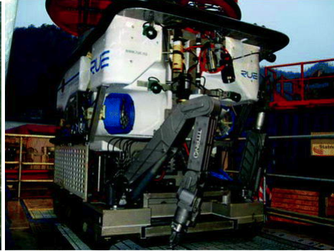
(b) ROV with grip manipulators and cameras (Worzyk 2009)
