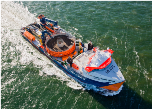
(a) Cable Laying Vessel (Nexus; Von Oord)
