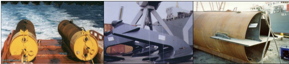
Figure 4.7: From left: Pile anchor (suction caissons); Anchor plates (DEA); Direct embedded plate anchor (SEPLA) (Diaz et al. 2016)
