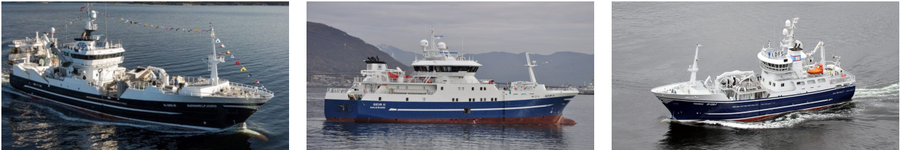
Figure 2.10: Illustration of three typical fishing vessels. Bømmelfjord, a pelagic trawler on the left, the autoliner Geir II, and the purse seiner Fiskebas (Eidesvik Havfiske, 2020; Baltic Shipping, 2019; Fiskebas, 2019).
