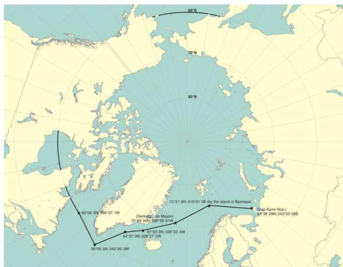
Figure 2.5: Maximum extent of Arctic waters. Adapted from International Code for Ships Operating in Polar Waters (p. 9) by IMO, 2017. Retrieved from http://www.imo.org/en/MediaCentre/HotTopics/polar/Documents/POLAR%20CODE%20TEXT%20AS%20ADOPTED.pdf . Copyright 2019 by IMO
