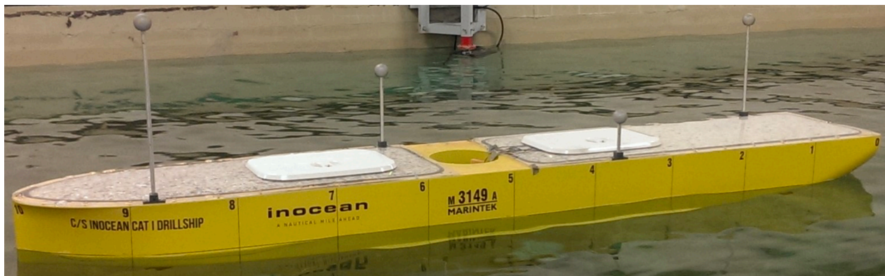
Figure 26: the CSAD, a 1:90 model ship of the Inocean Cat I Arctic Drillship (Bjørnø (2016))
