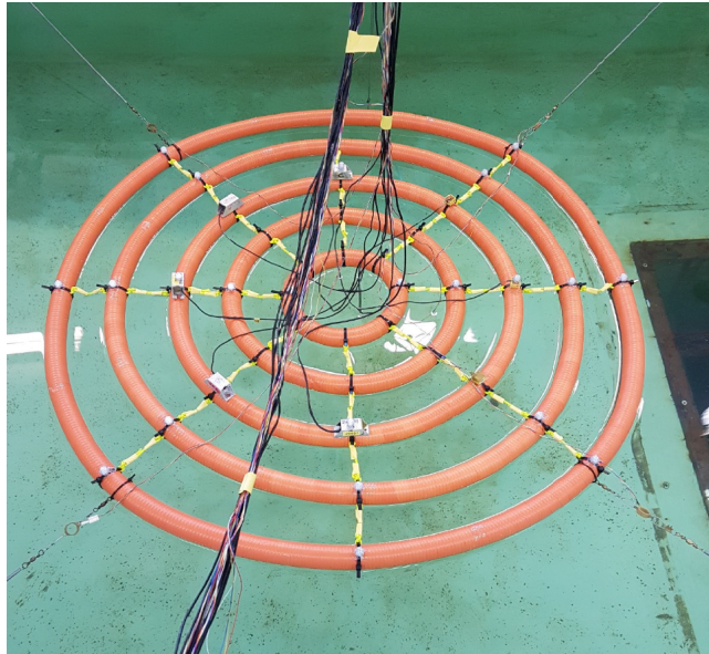
Figure 5.1: Multi-torus model by Winsvold Multi-torus model with instrumentation and mooring-lines. Grey, round reflexive markers as well as rectangular accelerometers are seen. Taken from Winsvold (2018).
