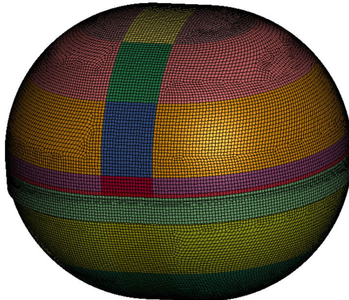
Figure 53: Meshed Model With Different Thicknesses
