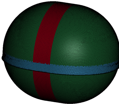
Figure 45: Boundary Conditions for Horizontal Tank
