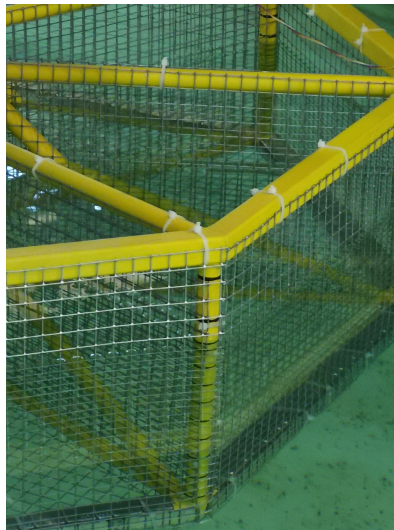
Figure 5.6: Close up picture illustrating the use of cable ties for fastening of the nets.
