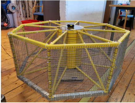
(a) Model with nets, after being painted and ballasted (b) Model without nets, before ballasting and painting
