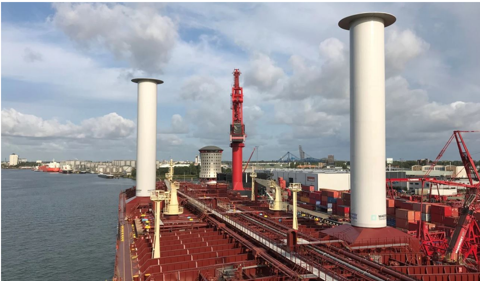
Figure 3.11: Flettner Rotor Installed on Mærsk Pelican Tanker. (Norsepower, 2019)
