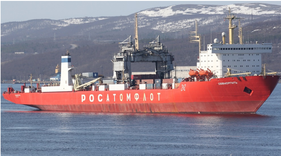
Figure 3.12: Sevmorput Nuclear Powered LASH vessel. (Norsepower, 2019)
