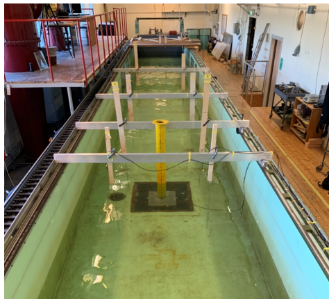
Figure 3.1.1: Photo of model test lab set-up. The wave maker is seen in the end of the tank.
