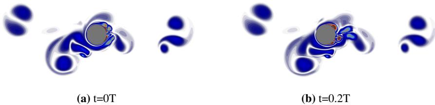
Figure 6.4.1: Vorticity at the surface for H_1/\lambda = 1/25 , T=1.73 .
